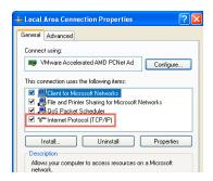
Under the Internet Protocol Properties, change the selection from "Obtain an IP address automatically" to "Use the following IP address." In the IP address, set it to 192.168.1.100 and the Subnet mask to 255.255.255.0. Click Ok to apply the settings, and then click Ok again for the previous Properties window.
