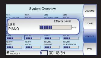
All channels in a myMix system can be named - mixing is as simple as selecting the instrument or vocal mic, press the button and adjust: volume, tweak the tone, add some effects and pan the signal within the stereo image. All settings, including the 4 band master PEQ are automatically stored in the current profile. 20 profiles are available to simplify operation. myMix lets you enjoy your music more.
