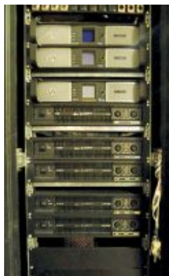
Clair Brothers PLM10000 and PL340 amplifiers power the FOH and monitor systems
