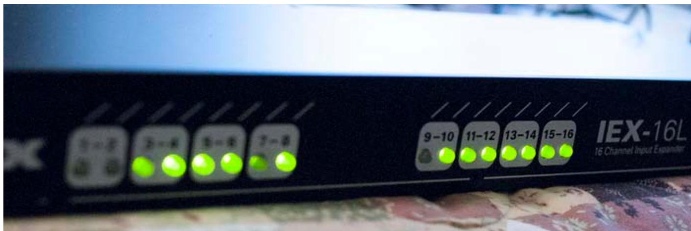
*THE BIG GREEN LIGHTS MAKE IT EASY TO SEE SIGNAL FLOW INTO THE A/D CONVERTER.*
