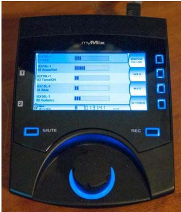
Each myMix mixer also has two XLR/TRS combo jacks on the back. These are inputs, that can be used for each musician's channels, and/or sent out to the network. One model for use is to have each musician plug their instruments into the myMixers, then everyone on stage can select from everyone's inputs. A "FOH" mixer could be used to dial up a house mix. In this set up, you wouldn't even need an input module. It also assumes you're not mic'ing the full drum kit with 8-10 mic's.
