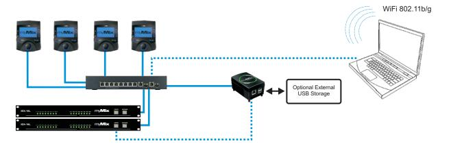
The myMix PLUG interface is connected to the myMix network directly on a switch or through the configuration port of an IEX16L input expander. The access to the myMix PLUG web server is either through WiFi or connecting the client interface to the Ethernet Network.
