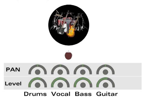
Pic 2: a mono mix means feeding the exact same signal to booth ears. This results in a one dimensional sound image with several consequences.
