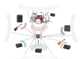
Pic 1: on stage we hear the backline and monitor speakers as well as the reflections from the stage and the house pa system: a true 3-D sound image with localization and room information.
