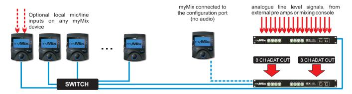
myMix and IEX-16L are connected to a managed Fast Ethernet switch (e.g. POWER8). Analogue inputs can be fed via IEX-16L and/or the local myMix inputs . Digital inputs can be fed via IEX-16L with ADAT Inputs (IEX-16L-A).
