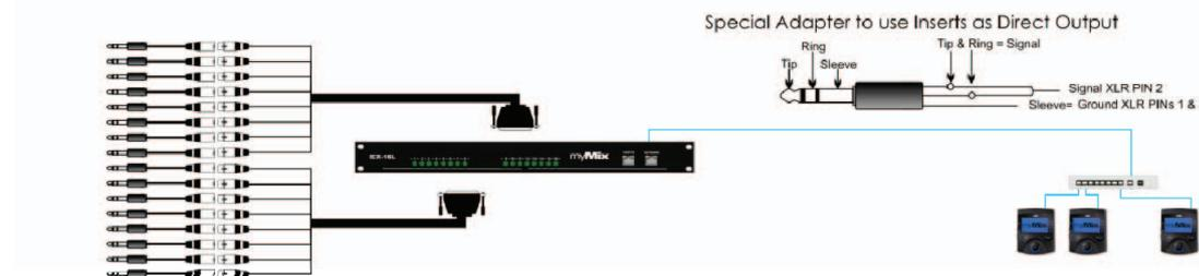
**Splitting Microphone Signal using a central Microphone Split and IEX-16L with external Pre Amps**
