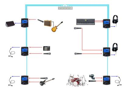
Audio sources are connected directly to the local inputs of myMix, without using a mixing console.
