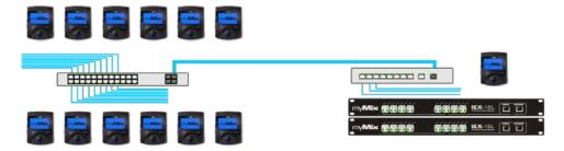
More than two switches get connected to a central GB switch
