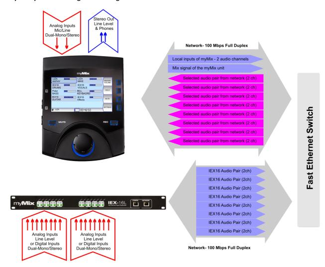
Each myMix has two local inputs for microphone for line level sources. They are streamed to the network and can be selected by every other myMix. The mix signal output is available as analog line level and headphone output and also selectable to be send as a network signal. This stereo mix signal can be selected from other myMix devices and used like all other input signals.
