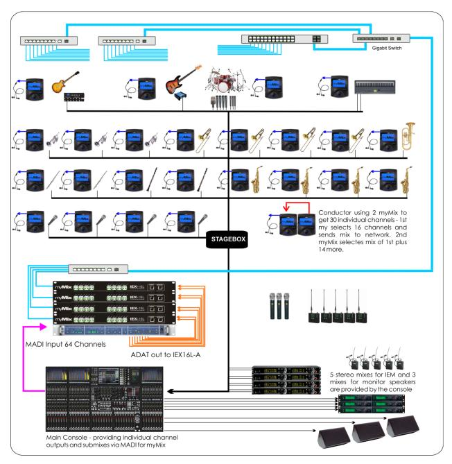
Large set up with dedicated monitor console. The monitor mixes for the solo artists are provided from the monitor console. Sub mixes and all individual instruments – up to 64 audio channels are send to the myMix system using a MADI signal via an RME ADI-648 interface to 4 IEX16L. The 64 channels in the network allows everybody in the band to select individual channels including the own instrument combined with some sub mixes.
