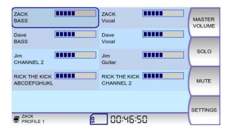
Each channel that is selected for the mix can be edited by moving the with encoder button to the channel and press it. The first parameter that comes up is the volume control, as this is the most needed parameter. Other functions are available via the soft keys on the right side. These include a tone control ß adding bass or treble to the signal, the stereo effects send for a 3D sound image, and panorama )or balance) for the positioning. Solo and Mute are available directly from the main screen.
