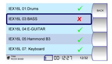
The channel counter on the right side of the control bar is showing the amount of selected channels and the amount of currently available audio channels on the network. Because of the audio streaming in pairs this indicator is only showing even figures.
