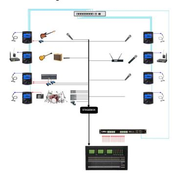
Submixes are fed from the console to an IEX16L(A), some direct inputs on stage are used in addition.
