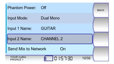
The IEX16L has 8 dual inputs for line level sources, which can be configured as dual mono or stereo channels and named like the channels on myMix. The IEX16L-A has additional digital, optical inputs in ADAT® format.
