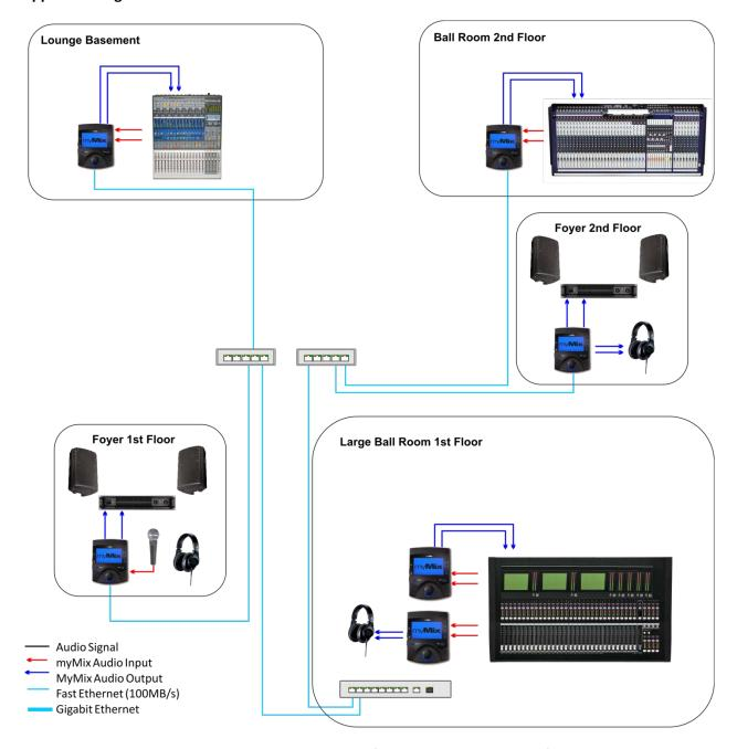
The easy CAT 5 connection allows to network signals from several stages easily for portable set ups. For longer cable runs a switch can be used as repeater.
