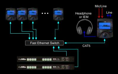
Each myMix unit has two mic/line inputs and the outputs for the stereo mix signal (headphone & balanced line level). They are connected to a conventional Fast Ethernet switch via CAT5 cable.
