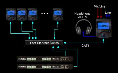
Each myMix unit has two mic/line inputs and the outputs for the stereo mix signal (headphone & balanced line level). They are connected to a conventional Fast Ethernet switch via CAT5 cable.
