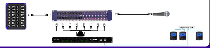
Using the Multicore Return for an Input from the Main Console to myMix
