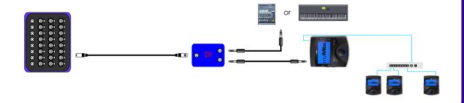
Splitting Microphone Signal for myMix and Main Console using a Mic Split Box
