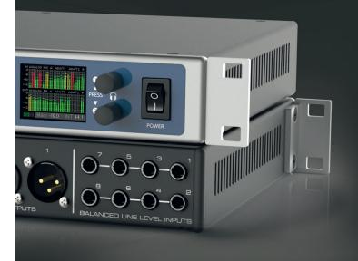
All new AD/DA converters, optimized analog I/O circuits, as well as improved SNR and THD values guarantee pristine, crystal clear and transparent audio. A new PAD-free mic circuit design with +18 dBu maximum input level and 75 dB gain range serves even the most critical recording situation and source trouble-free.
