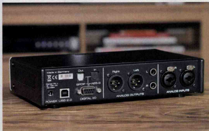
Photo 2: The ADI-2 Pro has XLR and optical S/PDIF inputs and outputs on the back.
