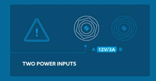
Dual redundant power supply inputs, with an on screen alert whenever one of the power supplies have failed.
